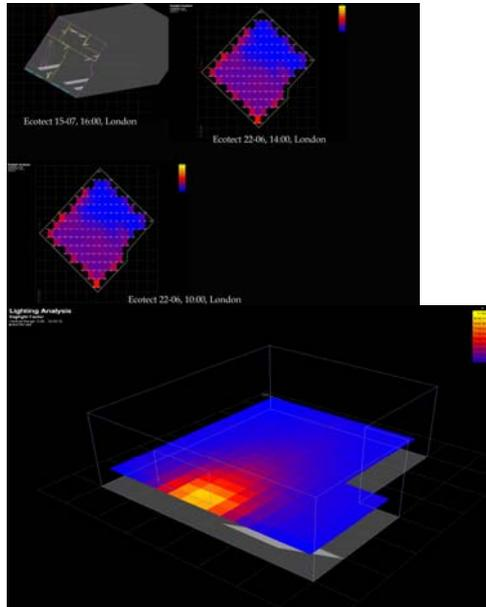
Figure 4.5 Ecotect Simple Daylight Factor Analysis
