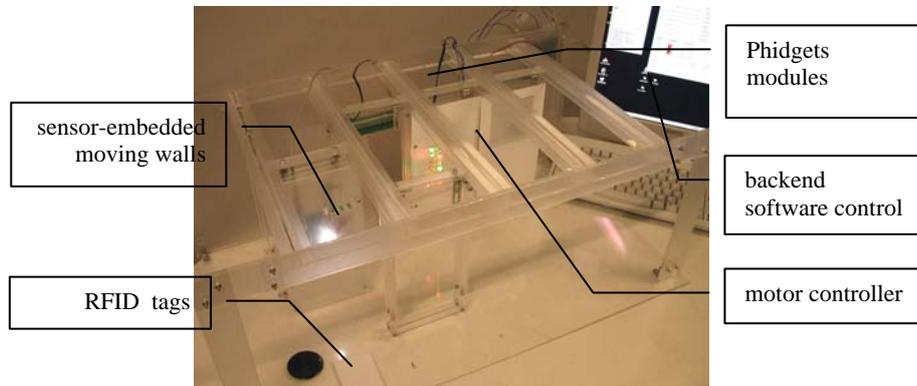
Figure 2. The sensor-based physical model serves as a medium for explicit representation of interactive moving partition wall system.
