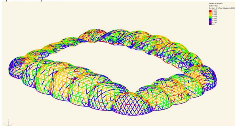
Figure 4. Stadium roof stress distribution diagram.
