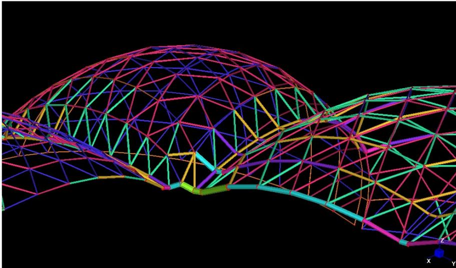
Figure 5. Detail of roof, optimized member sizes.
