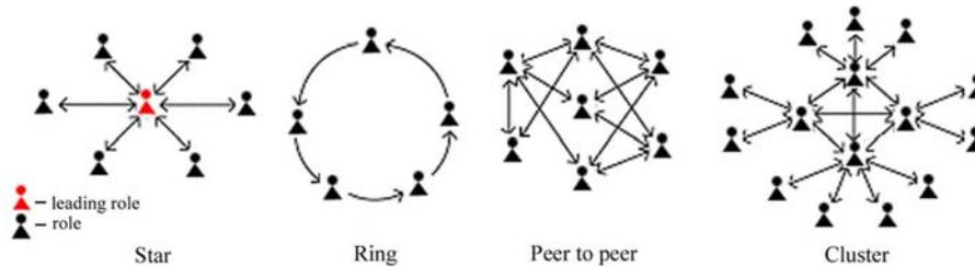
Figure 2. Four network topologies: star, ring, peer to peer and cluster
