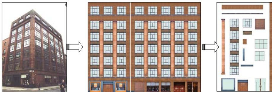
Figure 1: Creation of image map façades of individual building and disintegration of building to its elements
