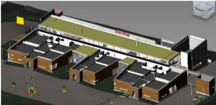
Figure 3. Architects Revit-model of the Kindergarten project “Toivo”. Design elements and components were extracted from Revit and imported to Klara cost estimation software via Excel-files, where cost estimation data was first sorted and organized.
