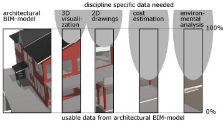
Figure 4. The usability of elementary architectural model. BIM-models always need additional domain specific data when they are used for various purposes.
