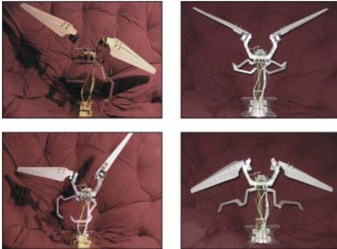
Figure 6. The Mimosa prototype alters its shape corresponding to the sun's position. The views of the prototype are mapped to the example design scenario (Figure 1).
