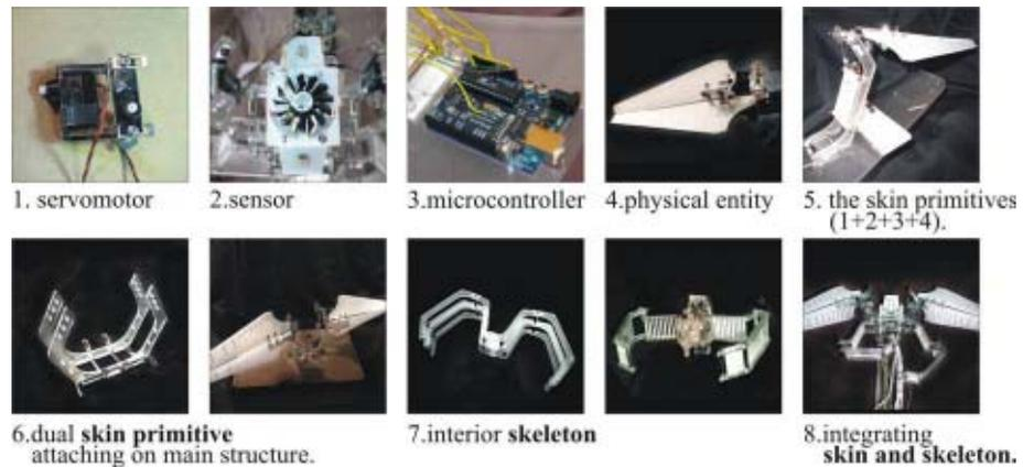
Figure 5. The development process of physical prototyping
