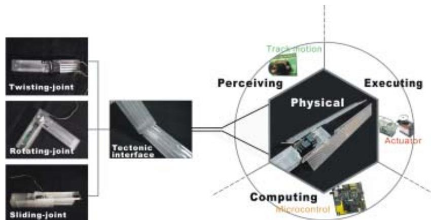
Figure 2. Three kinds of primitives (twisting joints, rotating joints, and sliding joints) are designed with tectonic interface; each of which can perceive, compute, and execute to adapt to change.
