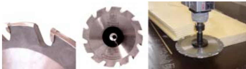
Figure 7. A disk shaped tool made of a regular saw blade.
