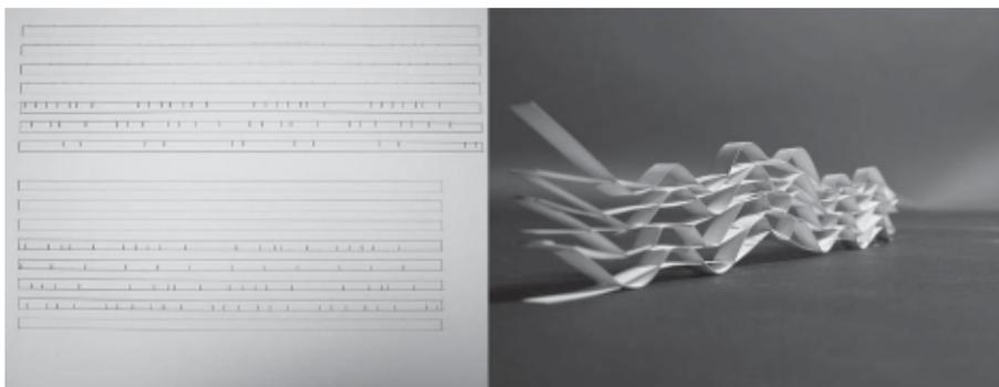
Figure 7. Physical Pattern Parts and Assembled Pattern Model: The authors created this pattern using the [SIN]uous system and a laser cutter
