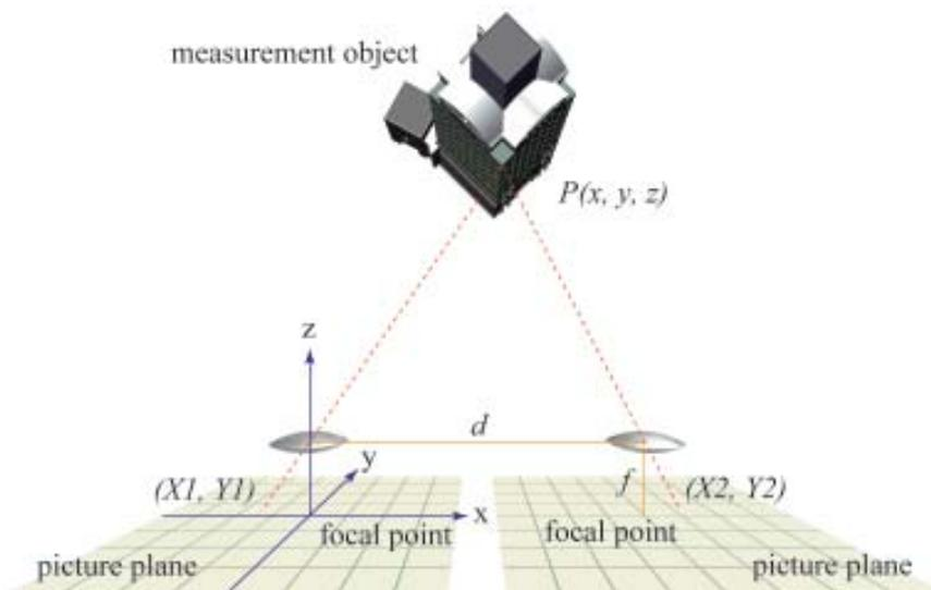
Figure 2. Basis of photogrammetry.
