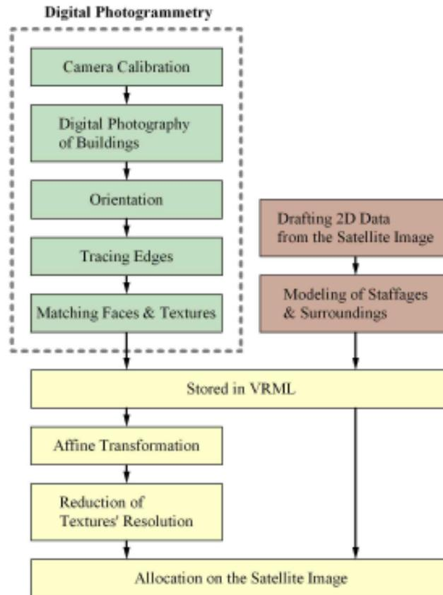
Figure 3. Process of constructing 3D urban models.
