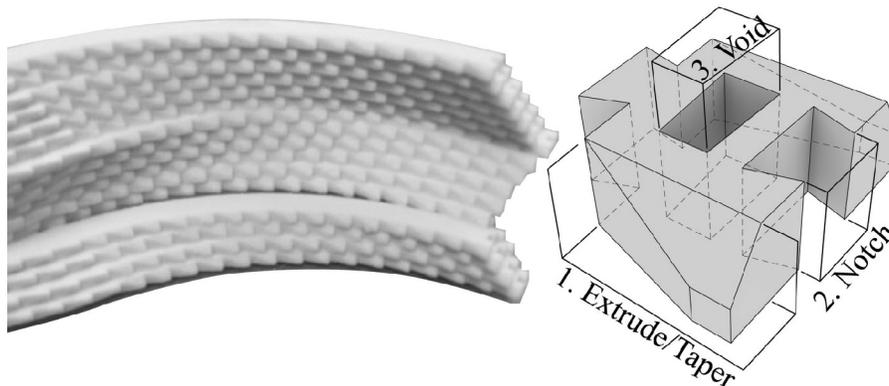
Figure 2. Studies of Masonry Module, development and combination.
