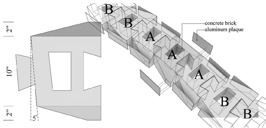
Figure 3. Masonry Module—dimension, shape, and connection. BBAAABB connection illustrated.
