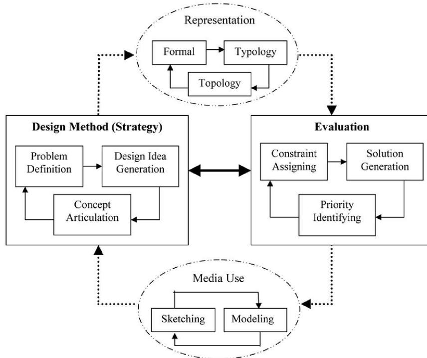
Figure 1. The cognition model of conceptual designing, showing its iteration loops and the two proposed external factors of media use and representation.
