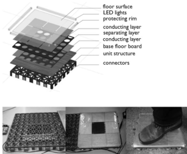
Figure 7. The detail design and prototype of Sensible Floor Tile (first prototype by Chi-Chieh Huang)
