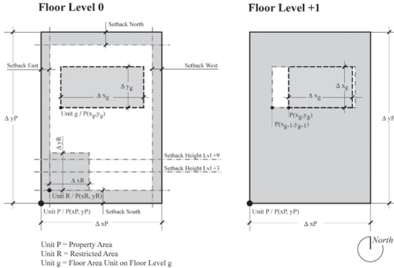
Figure 1. Area units per floor, their location on the ground floor and the following upper floor level.
