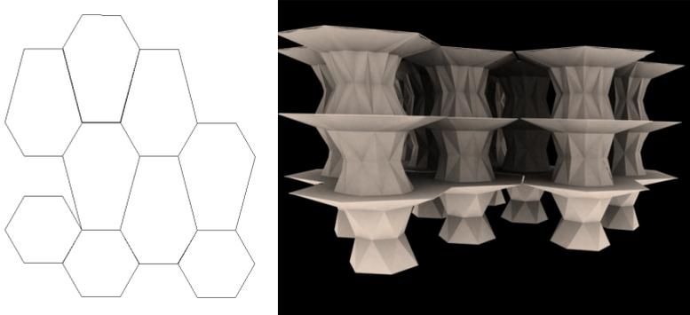
*Figure 3. Model of the pre-cast concrete units and plan.*
