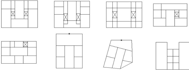
Figure 2. The top four images show digitisation of Palladio's villas, the lower four are computer generated variations using the schema.
