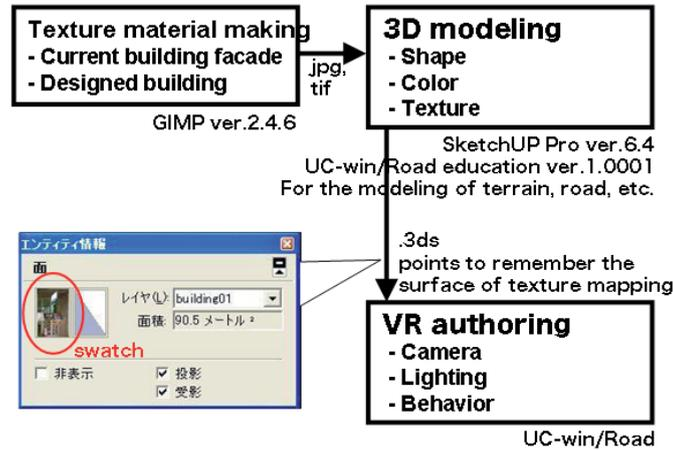
Figure 1. Developed use flow of 3D CAD / VR software.
