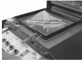
Figure 7. Vacuum forming process with MDF mould fabricated by CNC routing.
