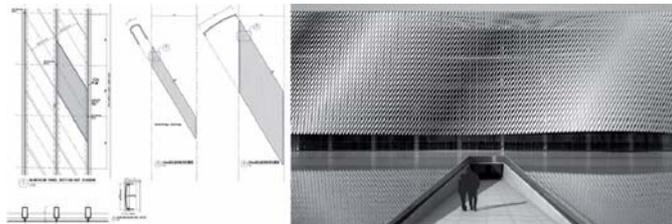
Figure 3. Folded profiles and the gradation pattern of the shading fins.
