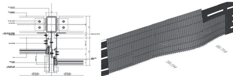
Figure 5. Deviation between glass unit and the design surface, and the corresponding mullion design to absorb the vertex offset.
