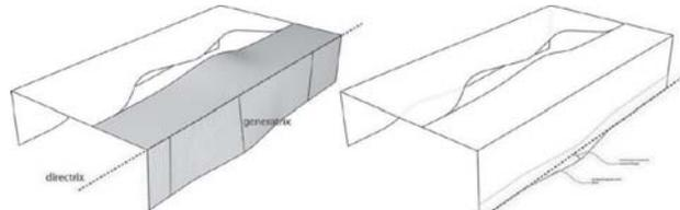
Figure 2. The definition of the ruled surfaces and the control of bulged surface.
