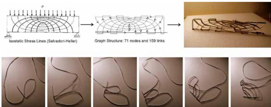
Figure 8. Stress lines as interwoven surface and assembly process
