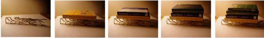
Figure 9. Load testing on the interwoven stress lines
