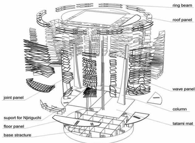
Figure 5. Axonometric drawing shows composition of parts.
