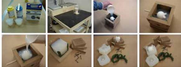
*Figure 6: Mould making and casting process*
