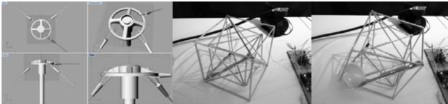
Figure 5. Digital detail of elastic joint that minimise friction (left); Physical *Cube* structure with sensors and embedded pneumatic air balloon to detect proximity of surface until reaches its stable state (right).
