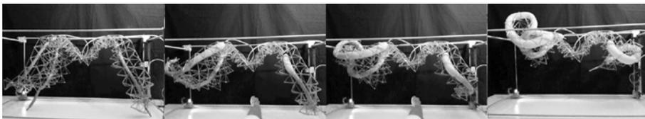
Figure 4. The Shelter contracts and expands in response to the proximity of human intervention and population through the pneumatic balloon as an elastic actuator.
