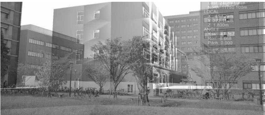
Figure 6. Actual field of view through the optical see-through HMD.
