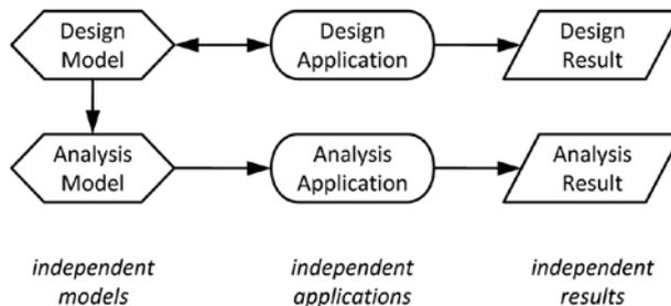
Figure 1. Data model interoperability: model exchange.
