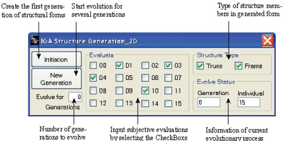
Figure 4. Panel for inputting evaluation and controlling evolution
