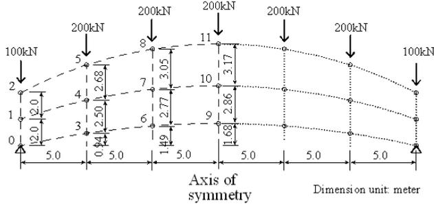
Figure 5. Designated node positions, load and support conditions
