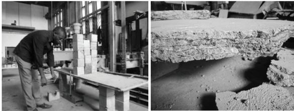
*Figures 6 and 7. Three-point bending test of panels for use in pre-cast assemblies.
