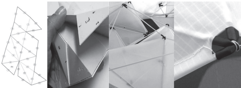
Figure 2. Unfolded cut pattern for TI mould (left). Laser-cut kite membrane and node.
