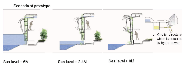
Figure 1. The kinetic structure is actuated by hydropower and changes its form according to the sea level.
