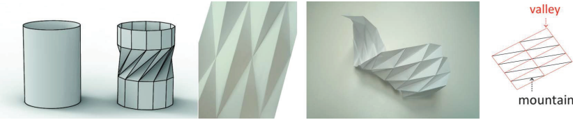
Figure 4. Diagonal Pattern as a result of cylinder torsion.
