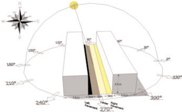
Figure 1. The idealized urban street scenario ( $h/w = 1:1$ ): showing the study areas of left and right pavements (each 3m) and the centre zone (9m) of a street and the six orientations.
