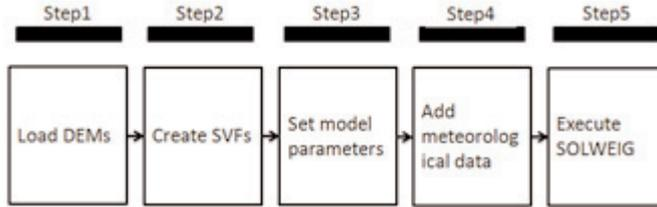
Figure 3. The five steps to simulate  $T_{mrt}$  using the SOLWEIG model.
