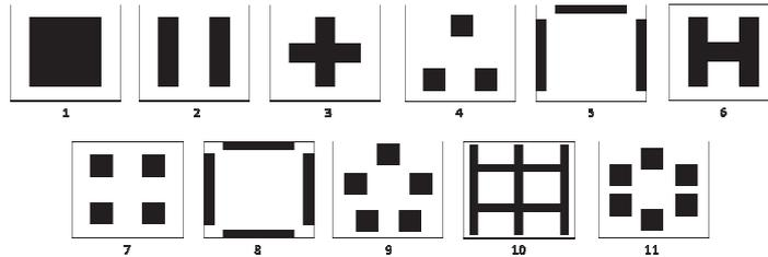
Figure 2. Eleven leg configurations are defined based on number and orientation of legs.
