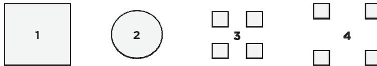
Figure 1. Test furniture area: cabinet (#1), dustbin (#2), stool (#3) and chair (#4). Roomba does not fit between the legs of the stool (#3), and it fits between the legs of the chair (#4).
