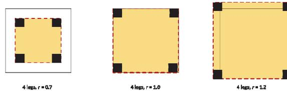
Figure 4. Three 'total area/leg area' ratio ( $r$ ) values are defined to capture leg coverage.
