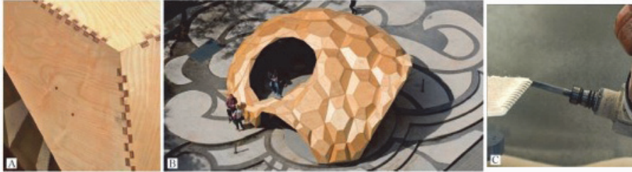
Figure 2: Robot fabrication of dovetail and Finger Joint of timber plates creating a shell structure (Krieg, O., et. Al, 2012)
