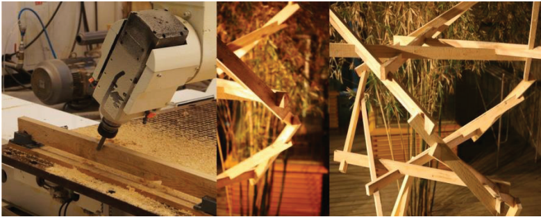
Figure 9. Rods milling with CNC (left); Junctions detail (middle); Connection between different layers (right).
