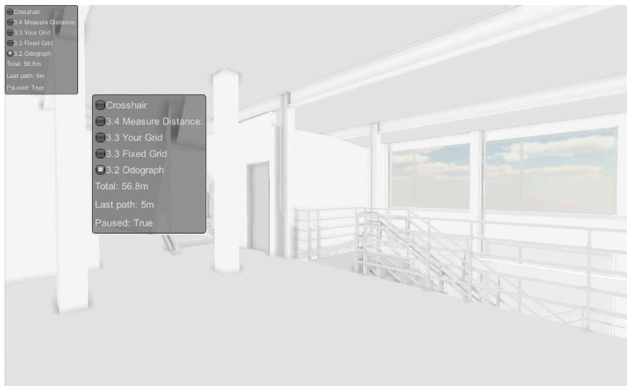
Figure 1. Odograph records and displays the user's total distance and last distance travelled, to allow correct comprehension of the scale of a building.
