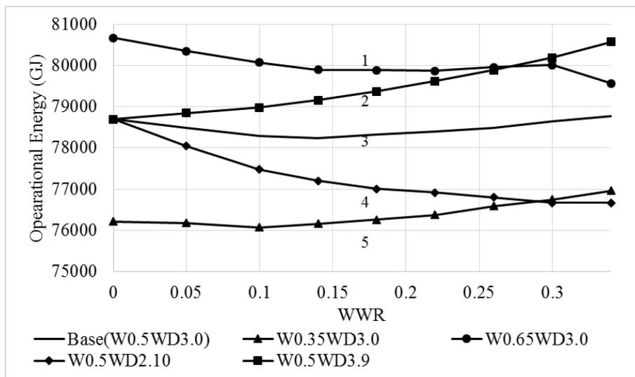
Figure 4. The variation of OE with WWR with respect to change in U-value of walls or U-value of windows.
