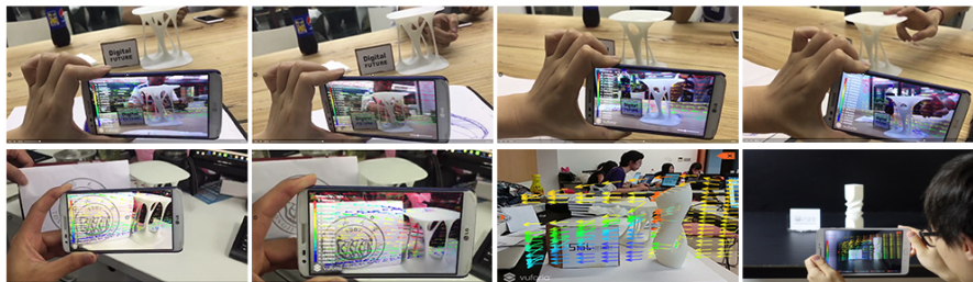
Figure 5. Wind environment visualization based on AR technology.
