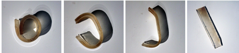
Figure 5. Initial test of SMP responsiveness: (a) the deformed shape of a fabricated polymer sample after applying heat and pressure, and (b, c, d) the shape recovery process at 2 seconds, 6 seconds, and 8 seconds.
