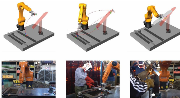
Figure 3. These images detail the robotic process of moving metal from pick up point to cutting jig and to assembly position for welding.
