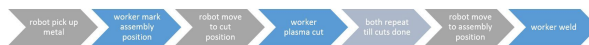
Figure 2. This diagram details the collaboration between machine and fabricator during the robot assisted assembly of the branching structures .
