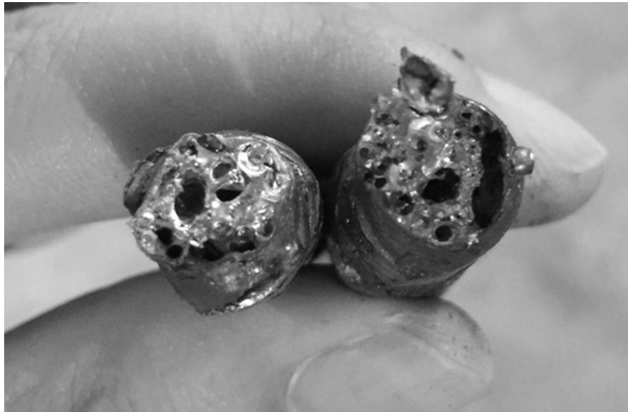
Figure 6. air bubble defects in the rods.
