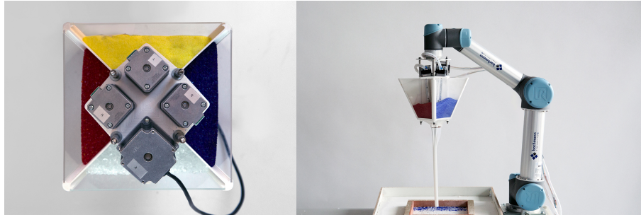
Figure 3. Top view (left) and elevation (right) of multi-channel tool and robotic setup.
