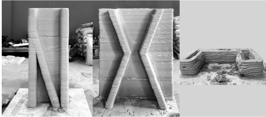
Figure 4. incline angle test 15°(left),20°(middle),25°(right).
