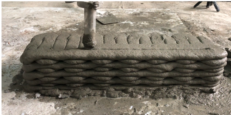
Figure 5. 90° cross pattern of test sample.
