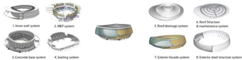
Figure 2. Eight systems for the hybrid building
