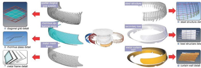
Figure 3. Exterior curtain wall system of the stadium
