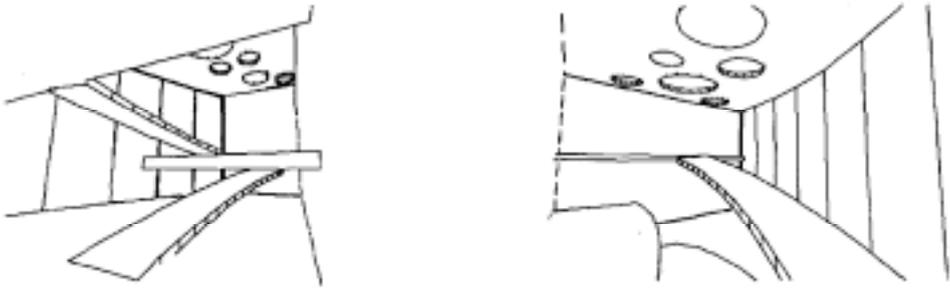
**Figure 19.** The relationship between the ramp and the openings in the ceiling that allow light to penetrate into the space.
