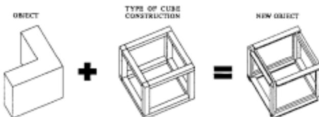
**Figure 4.** The function `CREATE-CUBE` creates a cube from a vocabulary type by instantiating it as the twelve edge elements.
