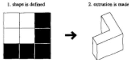
**Figure 1.** The interface used to create extruded objects.
