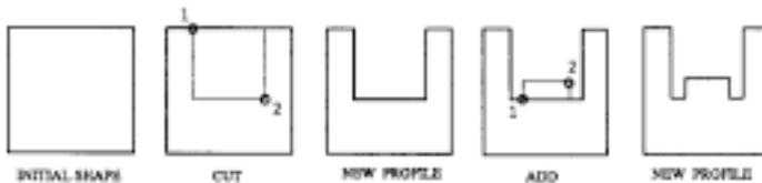
**Figure 6.** The interface to create two-dimensional profiles with cutting and adding operations.
