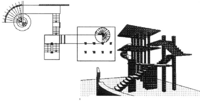
**Figure 17.** Creating a scheme with the structure and circulation systems. Project by Thomas Kaempfer.
