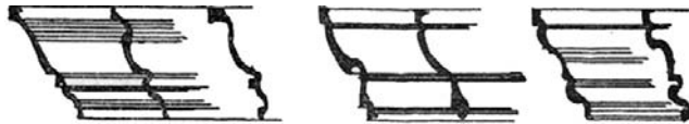
Figure 4. Classical profiles that have been digitally morphed by moving their control points (the original 'a' and new profiles 'd' and 'e' are shown here).
