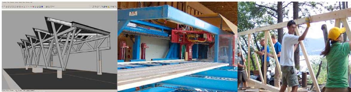
*Figure 2. Digital modeling, CNC fabrication, and assembly*
