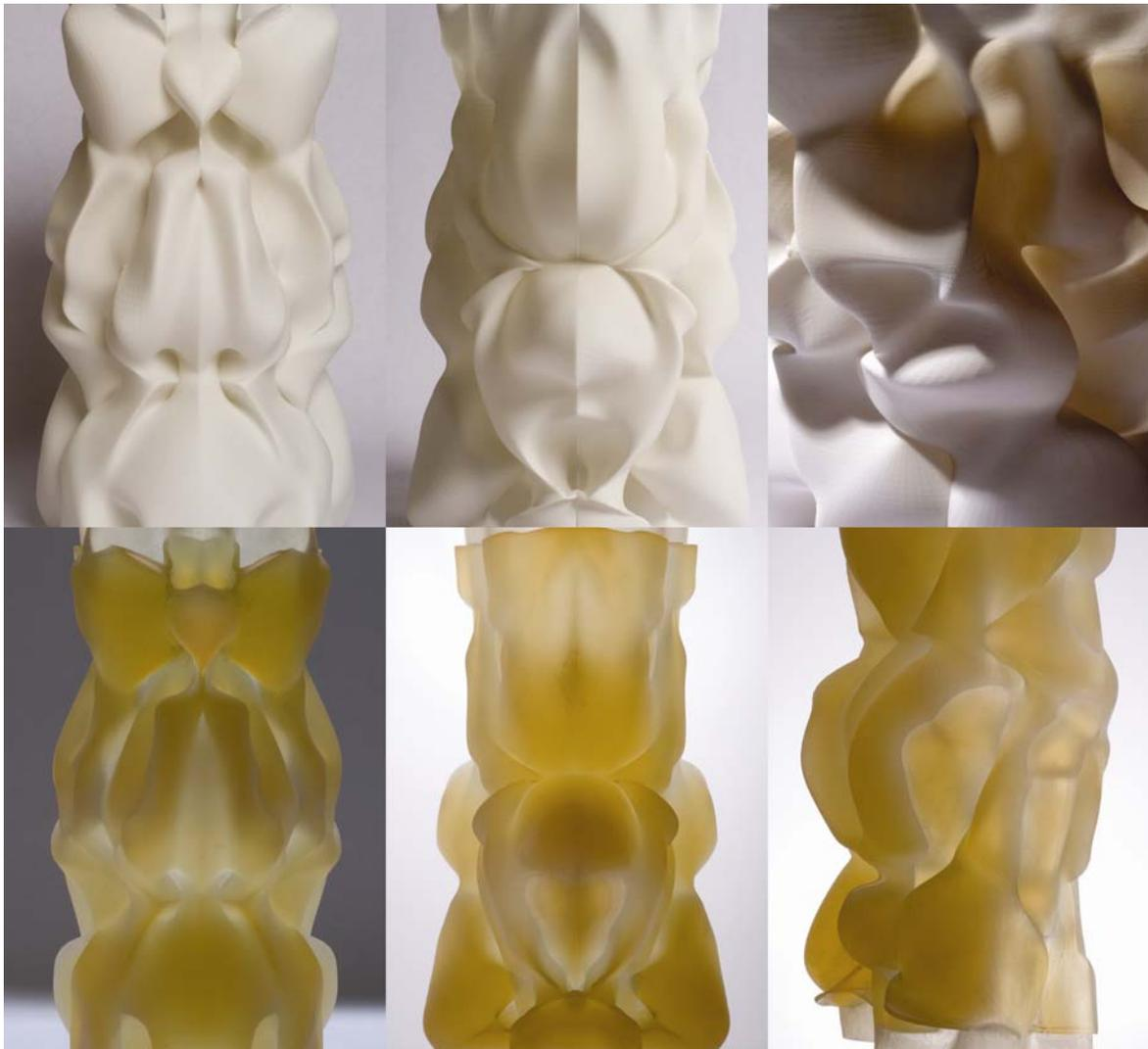
Figure 2. *Raycounting*: SLS nylon models (top) and printed resin composites including structural pockets (bottom).
