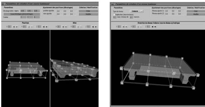
Figure 3 Dialog Boxes for the Creation of the Light Sources and Networks
