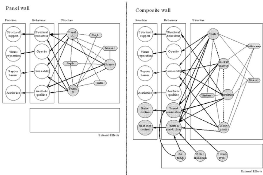
Figure 7 Comparison of the panel and composite wall FBS descriptions. Differences are shaded.
