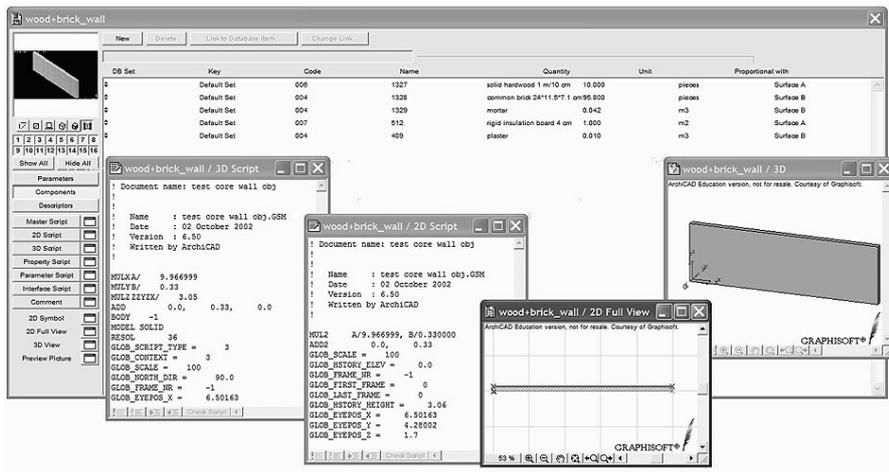
Figure 6 Composite Wall GDL Object
