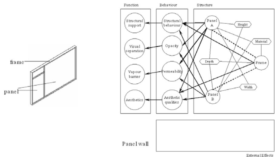
**Figure 1 A Panel Wall and its Corresponding FBS Representation**
