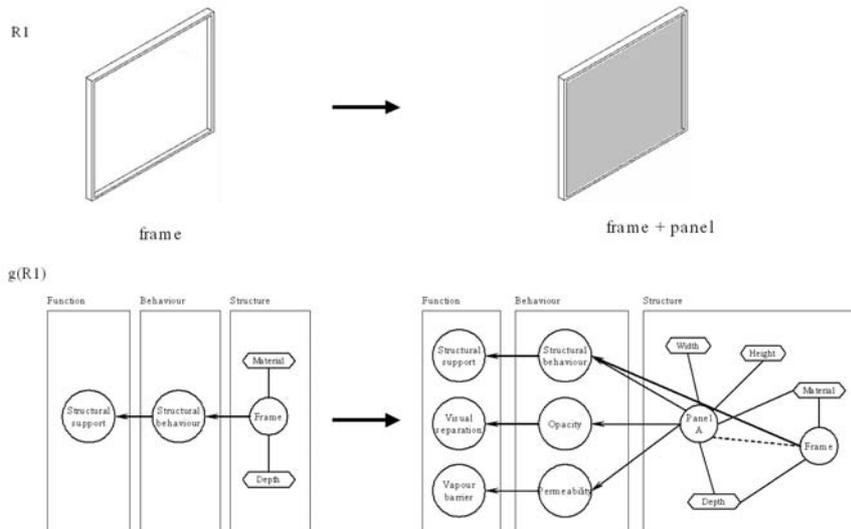
**Figure 2 A Rule to Generate a Panel Wall and its FBS Description**
