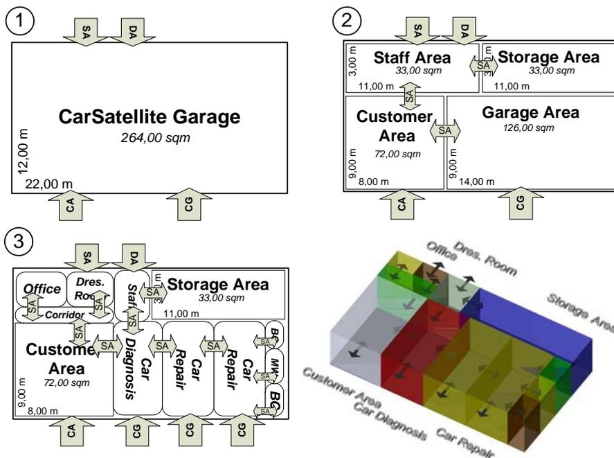
Figure 3 Conceptual Design Sketch with Top-Down Decomposition
