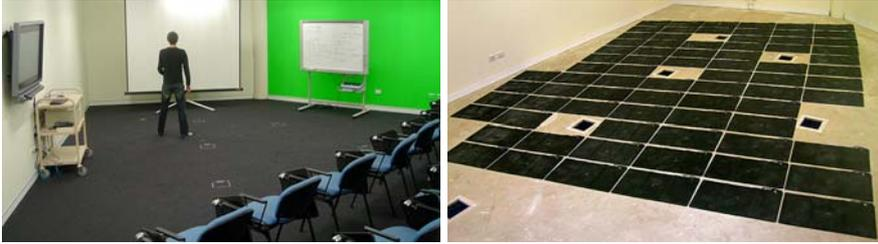
**Figure 1 The Key Centre of Design Computing and Cognition Sentient Lab showing “invisible” pressure sensitive floor mats embedded underneath the carpet, triggering the visual and auditory sound system and (right) before carpeting the grid of pressure mats laid on the floor, networked to the Teleo (MakingThings 2003) modules for conversion to a USB interface.**
